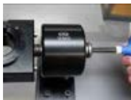
Optional: Assemble Tool Block Head to the Base by rotating the Push Knob on the back of the Base, Snug tighten with supplied 8mm Wrench
