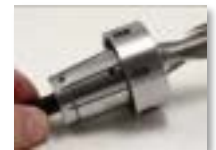
Insert the preset screw finger tight against the back of the cutting tool to hold the cutter in place and eliminate gap and movement
