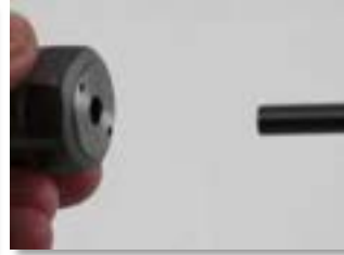
Insert cutting tool with the seal engaged on the round part of the shank, tighten cap.
