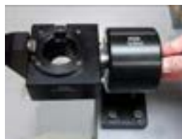
Push in on the Push Knob to unlock the head from the base
