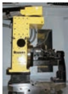
CNC401T is installed on the pallet of the horizontal M/C.
