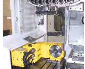
2 units of CNC rotary tables are used on the TAPPING CENTER with swing type pallet changer.
